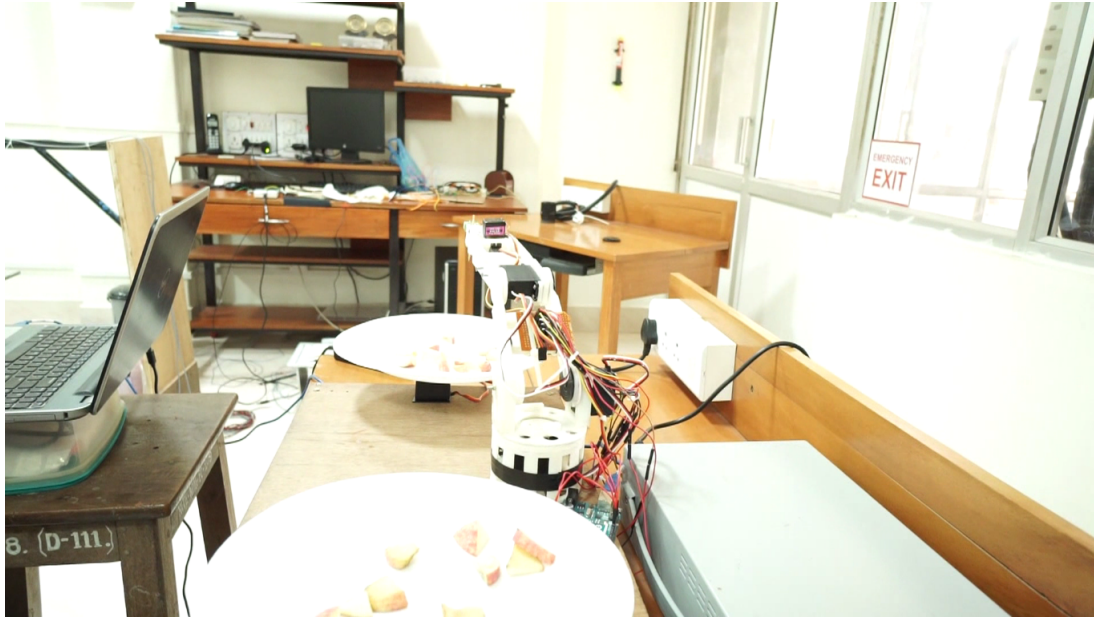
Figure 3.15: Robotic arm picking a fruit
